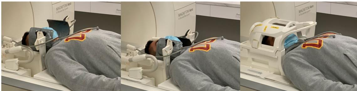
**Fig. 3** Custom upper airway (UA) and prototype head-neck (HN) coil for 0.55 Tesla MRI. (Left) 8-channel UA coil before adjustment of coil elements. (Center) UA coil with coil elements placed as close as possible to the upper airway region without contacting the skin or otherwise altering speech production. A 9<sup>th</sup> element can be placed in
